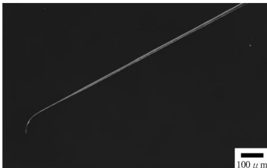
Figure 5 SEM image showing the tip appearance of a tensile fractured fiber at 1273 K, of an amorphous \text{Al}_{32.4}\text{Er}_{7.6}\text{O}_{60} continuous fiber made with melt extraction method.
